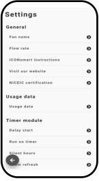
**Usage Data** — The iCONsmart can store up to 3 months rolling log of power use, time-on, flow rates, temperature and humidity levels (Requires the humidity module to be installed and connected to view temperature and humidity levels log).
