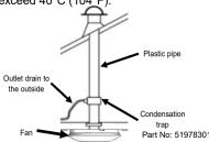
To avoid the backflow of condensation into the fan in ceiling installations Airflow recommends fitting a condensation trap to the outlet duct of the fan.
