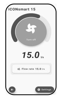
**Home** — From this page you can activate the fan, as well as viewing and adjusting the flow rate.
