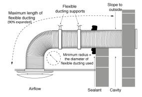
Ensure that flexible duct connections are not over tightened to the spigots. To maximise the air flow, rigid ducting should be used where possible. The fan and ducting should be installed in accordance with the requirements of the Domestic Ventilation Compliance Guide, part of Part F of the Building Regulations.
